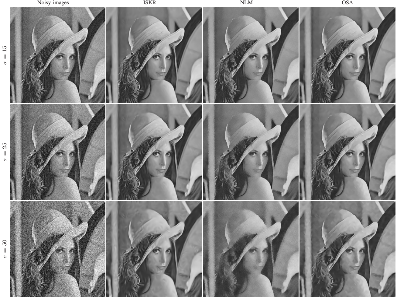
Fig. 1. Examples of white Gaussian noise reduction: The columns left through right show the noisy image and the restored images by ISKR [1], NLM [2], OSA [3]. The rows from top to down are showing the experiments with different standard deviations ( \sigma = 15, 25, 50 ). The corresponding PSNR values are shown in Table I.
