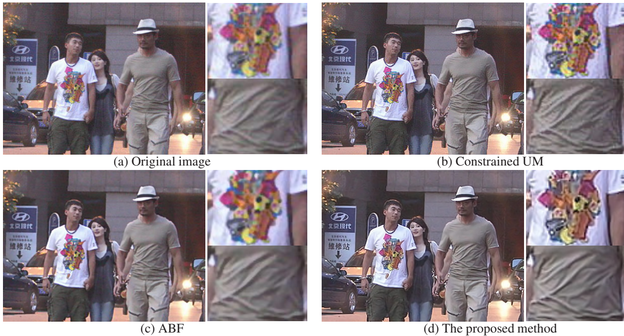
Figure 6. Experimental results of sharpening a weakly blurred and strongly noisy image. (a) input image; (b) result of Constrained UM [2]; (c) result of ABF [18]; (d) result of Proposed method.
