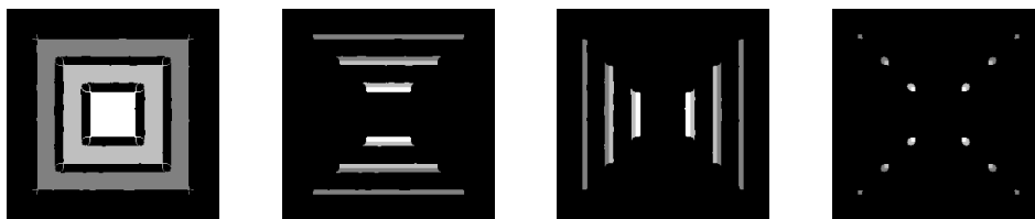
Figure 2.5: Clustering results by K-Means algorithm on the box image. Notice how edges and patterns of a certain kind are clustered together even though the patches may have different intensities.
