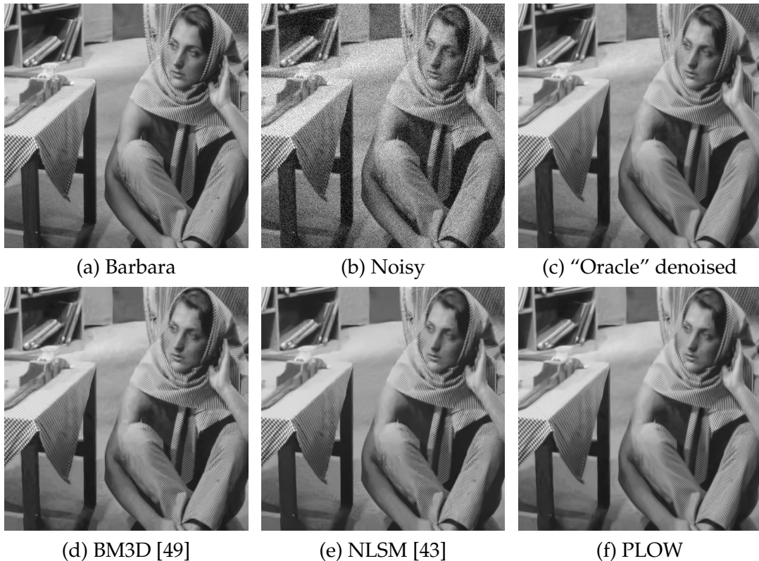
Figure 5.5: Comparison of denoising results for the Barbara image corrupted by WGN of \sigma = 25 . (a) Original image, (b) noisy input, (c) PLOW with “oracle” parameters (MSE 49.42), (d) BM3D [49] (MSE 56.17), (e) NLSM [43] (MSE 61.00), and (f) PLOW (MSE 62.64). High resolution images can be viewed at http://users.soe.ucsc.edu/~priyam/PLow/ .
