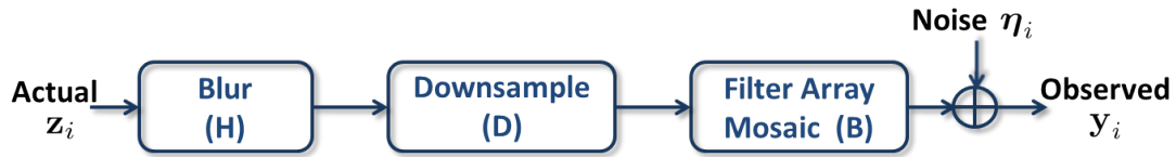
Figure 6.3: Image formation model showing the different degradation steps that the image goes through due to camera hardware limitations. The captured (raw) signal undergoes further in-camera processing before it is finally stored.
