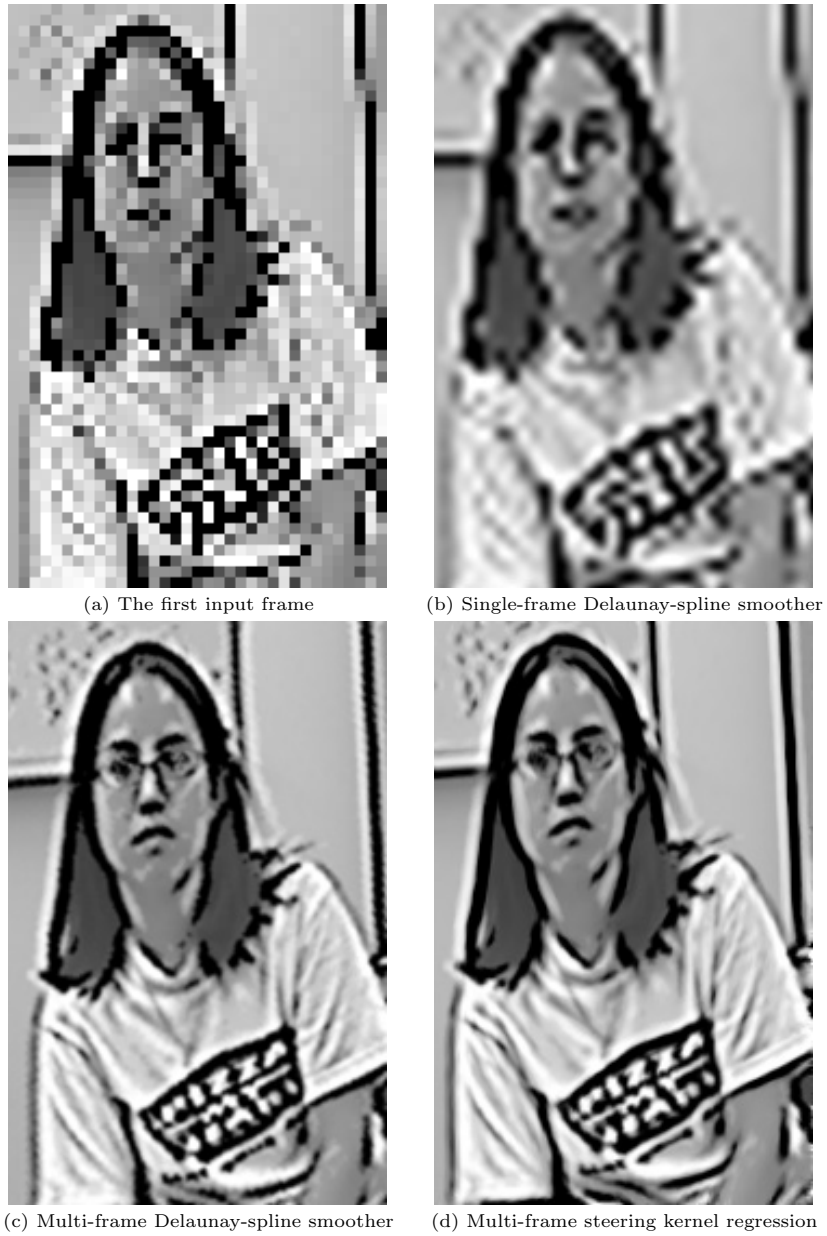
Figure 5.9: Image fusion (Super-Resolution) experiment of a real data set consisting of 10 compressed grayscale images. One input image is shown in (a) which is up-scaled in (b) by the spline smoother interpolation. (c)-(d) show the multi-frame Shift-And-Add images after interpolation by the Delaunay-spline smoother and the steering kernel methods. The resolution enhancement factor in this experiment was 5 in each direction.
