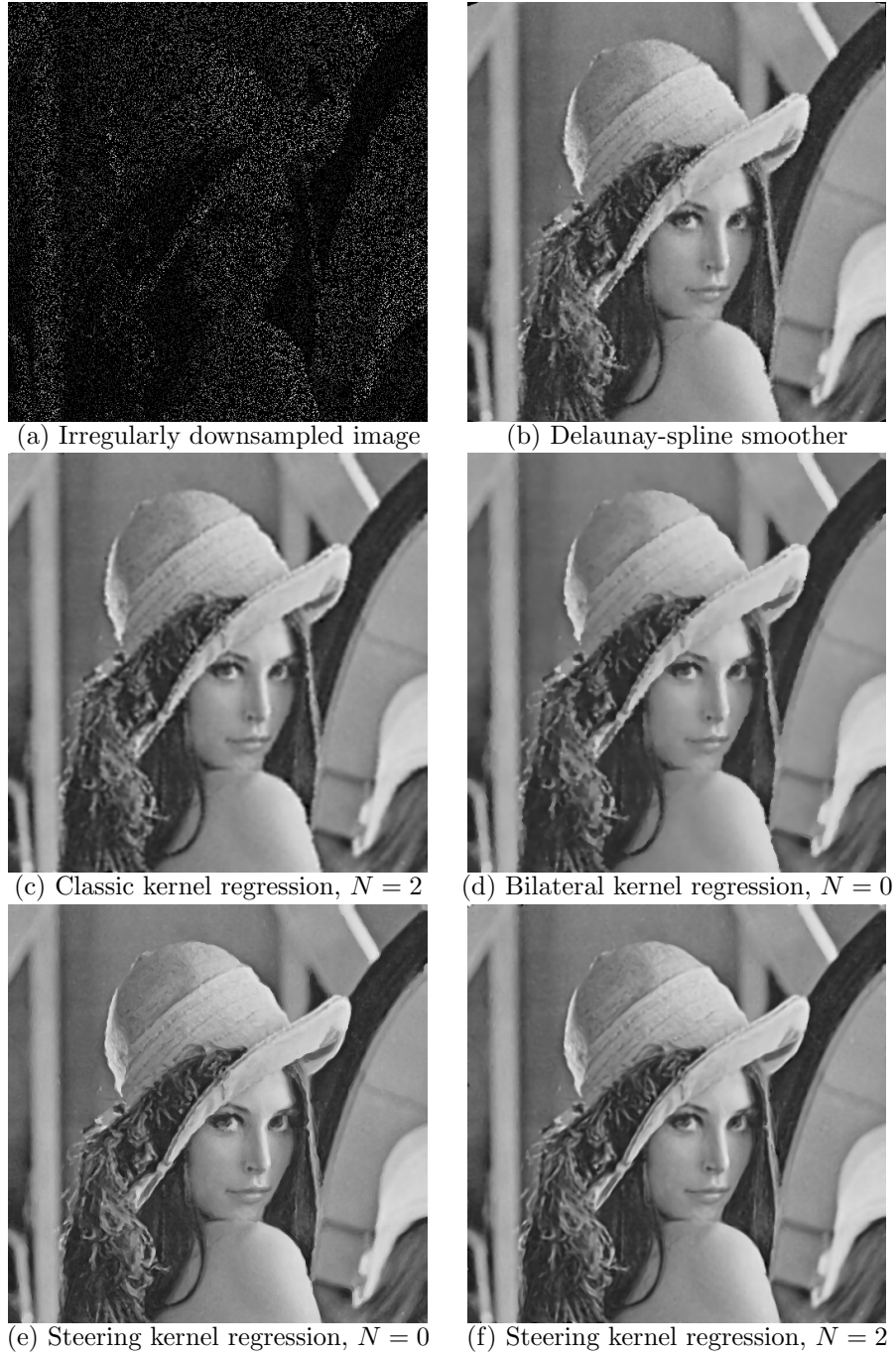
Figure 5.7: Irregularly sampled data interpolation experiment, where 85% of the pixels in the Lena image are omitted in (a). The interpolated images using different methods are shown in (b)-(f). RMSE values for (b)-(f) are 9.15, 9.69, 9.72, 8.91, and 8.21, respectively.
