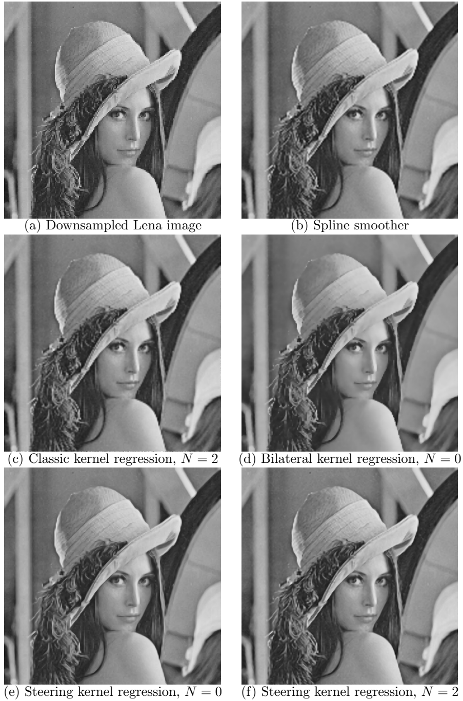
Figure 5.5: Upscaling experiment. The image of Lena is downsampled by the factor of 3 in (a). The factor of 3 up-sampled images of different methods are shown in (b)-(f). The RMSE values for images (b)-(f) are 7.92, 7.96, 8.07, 7.93, and 7.43 respectively.
