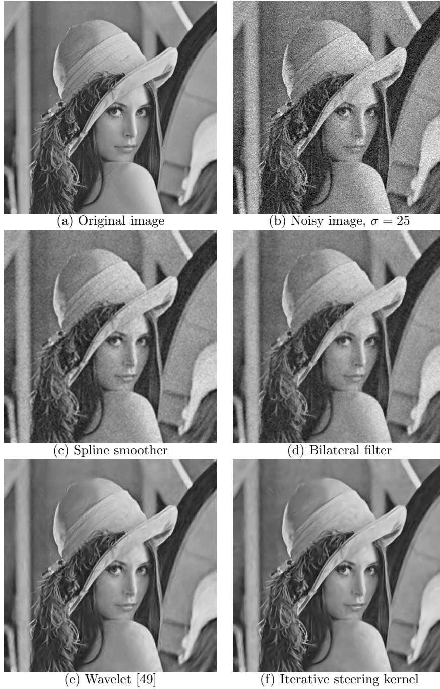
Figure 5.1: The performance of different denoising methods are compared in this experiment. The RMSE of the images (b)-(f) are 25, 8.91, 8.65, 6.64, and 6.66, respectively.
