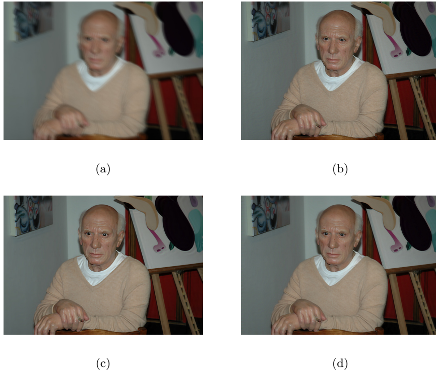
Fig. 2.11: Real motion deblurring example: (a)input blurred noisy image, (b)output of hyper-Laplacian algorithm [58], (c)output of [97], and (d)output of our algorithm ( \eta = 0.031, \beta = 0.6 ).
