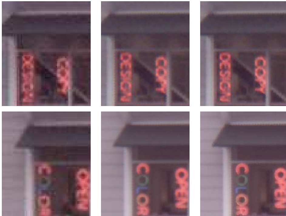
Figure 1.16: The images in the left hand column show frames #1 (top) and #69 (bottom) of the 74 frame low-resolution CFA image sequence. The second column shows the results after the recursive dynamic Shift-and-Add processing increasing their resolution by a factor of three in each direction. The right column shows the images after iteratively deblurring the dynamic Shift-and-Add images. We observe that the dynamic Shift-and-Add performs much of the work, while the subsequent deblurring restores the final details to the images.
