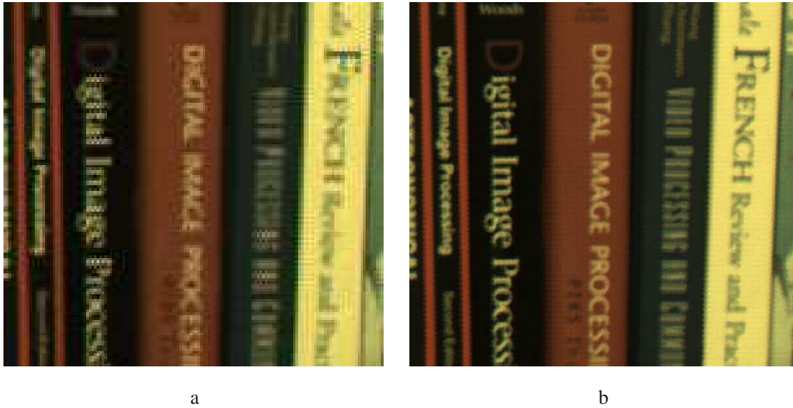
Figure 1.11: Multi-frame color super-resolution applied to a real data sequence. (a) shows one of the 31 low-resolution input images (of size [141 \times 147 \times 3] ) demosaiced by the single-frame method of [7]. (b) shows the resulting image after multiframe demosaicing using the robust data penalty term of (1.14). The resulting image shows improved resolution and reduced color aliasing artifacts (©[2007] IEEE).
