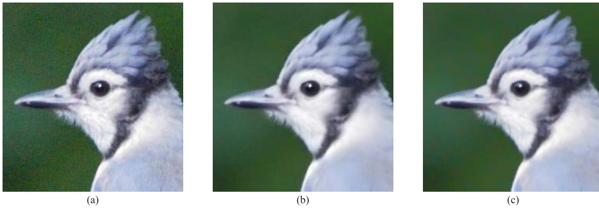
Fig. 11. Comparison of denoising performance on the real noise. (a) Noisy image, (b) Neat Image™, (c) G-NLM. (Neat Image™denoising software is available at http://www.neatimage.com .)
