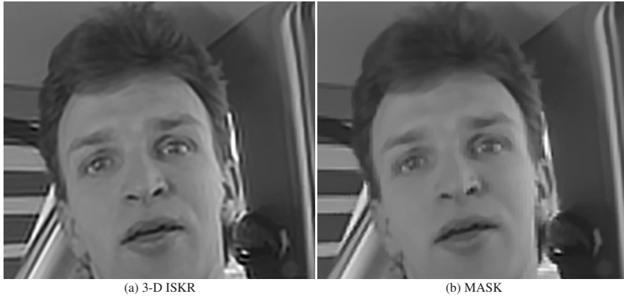
Fig. 12 Spatiotemporal upscaling of Car-phone video sequence: (a) upscaled frames by 3-D iterative SKR [24] at t = 25.5 , and (b) upscaled frames by MASK at t = 25.5 . In this example, we upscale Car phone sequence shown in Fig. 11(a) with the spatial upscaling factor 1 : 3 and the temporal upscaling factor 1 : 2.
