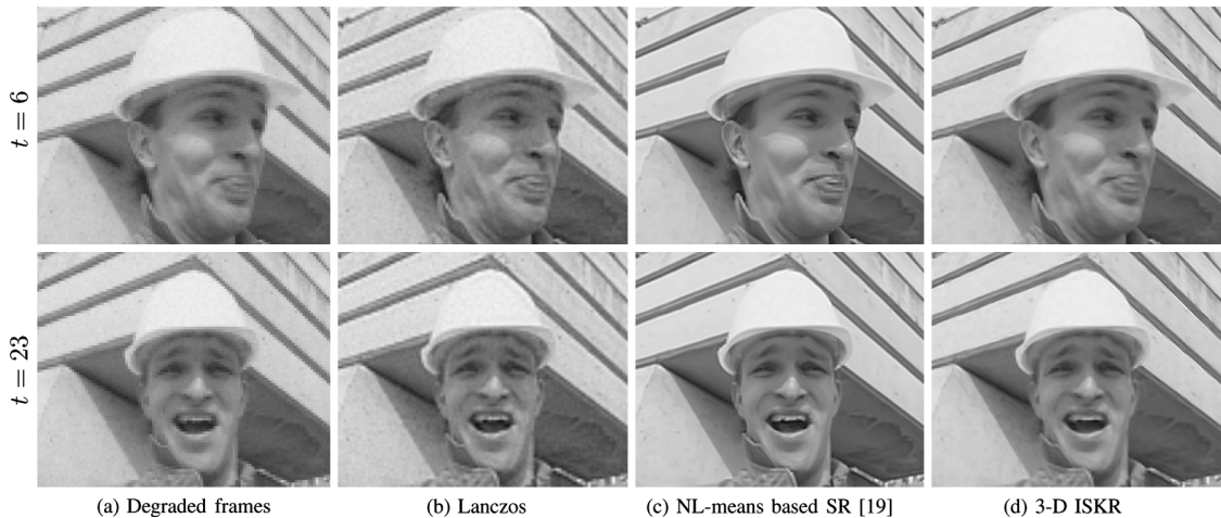
Fig. 9. Video upscaling example using Foreman sequence: (a) The degraded frames, (b) the upscaled frames by Lanczos interpolation [PSNR: 31.01 (top) and 30.21 (bottom)], (c) the upscaled frames by NL-means based SR [19] [PSNR: 32.13 (top) and 31.94 (bottom)], and (d) the upscaled frames by 3-D ISKR [PSNR: 33.02 (top) and 32.12 (bottom)]. Also, the PSNR values for all the frames are shown in Fig. 10(b).
