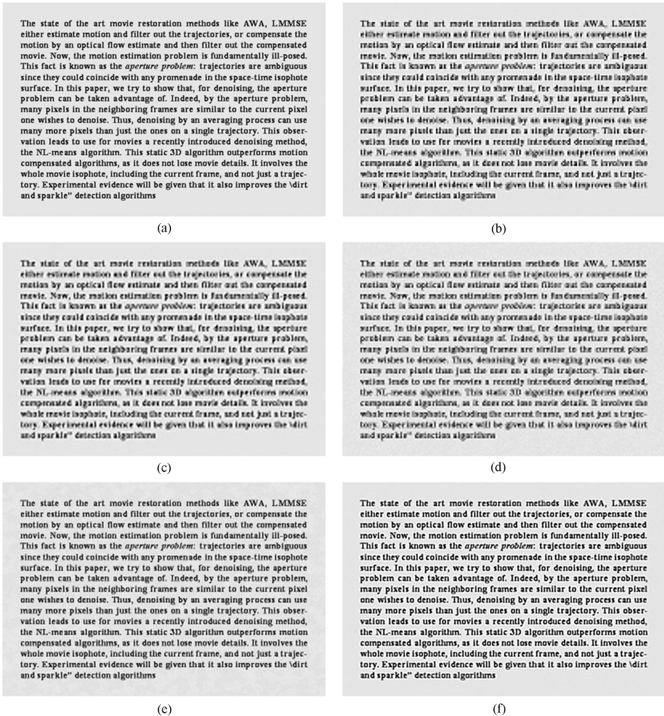
Fig. 6. Results for the synthetic text sequence. (a) Original (ground-truth) image. (b) Pixel replicated image, 13.47 dB. (c) Lanczos interpolation, 13.84 dB. (d) Deblurred Lanczos interpolation, 13.9 dB. (e) Result of shift-and-add algorithm [18], [20], 18.4 dB. (f) Result of proposed algorithm, 18.48 dB.
