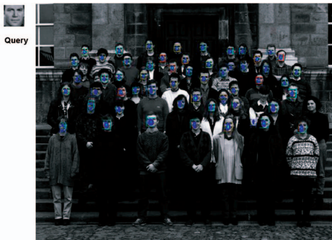
Fig. 18. Detection results on the MIT-CMU multiscale test set [54]. \alpha was set to 0.99. Among 57 faces present, we detected 54 faces at a correct location with four false alarms.
