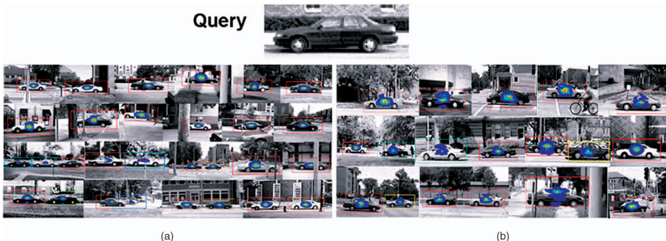
Fig. 13. (a) Examples of correct detections on the UIUC single-scale car test set [53]. (b) Examples of correct detections on the UIUC multiscale car test set. Confidence level \alpha was set to 0.99 and RM only above the threshold \tau corresponding to \alpha is embedded in test images. Bounding boxes are drawn at the correct locations. In case of a multiple detection, a red bounding box indicates higher resemblance to Query than a blue bounding box.
